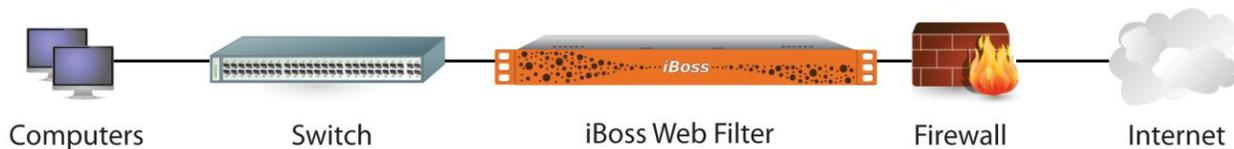
**Figure 7 - Inline Installation**
